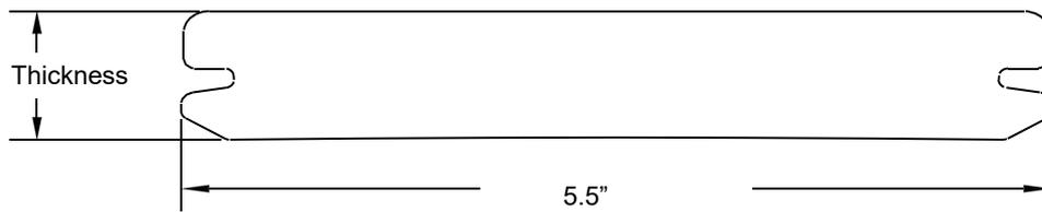
FIGURE 3—TREX® TRANSCEND G2 GROOVED-EDGE DECK BOARD PROFILES
