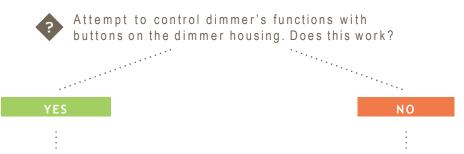
If your dimmer remote does NOT have a metal antenna, replace the dimmer or rely on housing controls.
