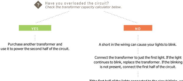
If the first half of the lights connected to the circuit blinks, work backwards checking each light. The possible short is likely in the first half of lights. If the lights do not blink while the first half is connected, go ahead and connect the second half of the circuit.
