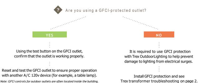
If the GFCI outlet is working, but the lights are not working, see Trex timer troubleshooting on page 2.
