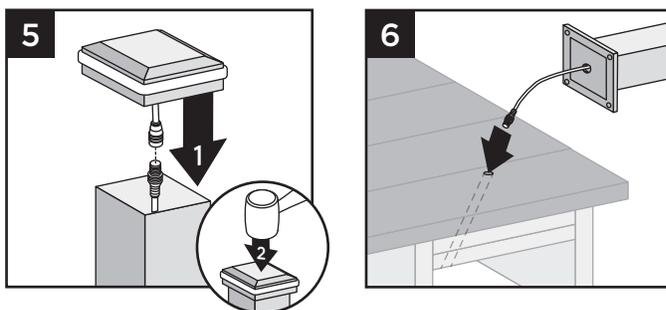
5. Connect the female connector on the post cap light to this wire and, using a rubber mallet, gently tap the cap onto top of post until it is secure.
