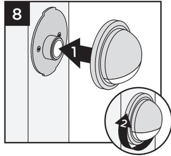
**NOTE:** If railing has already been installed, lead wires will need to be fished through the post sleeve to reach the desired location for the deck rail light. In some cases, if the provided lead wire does not fit (due to connector size), the wire connectors can be cut off and wire nuts can be used. Test lights with the power on. If lights that are wired with this method do not function, then switch the connector wires.
