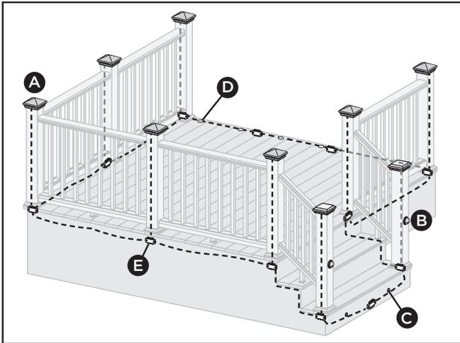
**NOTE:** All wiring and splitters are mounted to the inside of framing. Picture above is a general representation of where to place them.
