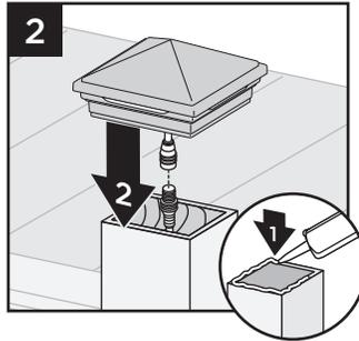
1. Connect male lead from wiring to female connector from cap. Also attach male-to-male connection wires in between each splitter. Continue until all wiring from lights is attached to splitters and connector wires are attached in between splitters. (See *Making Connections* section for details.)
