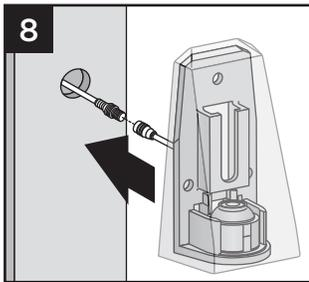
8. Connect male connector to female connector on light housing.
