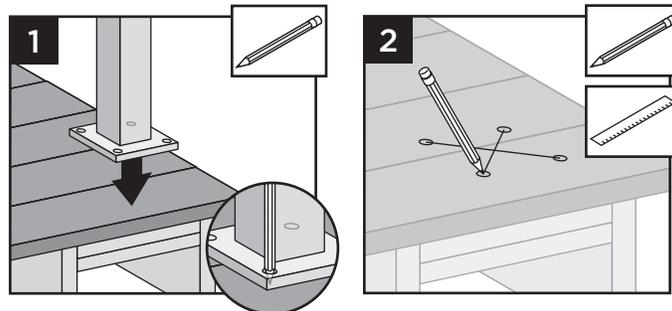
1. Before attaching post to deck, locate placement of post and mark desired bolt locations.
