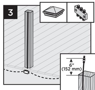
2. Wiring can be run under deck and behind risers. Staple to frame with cable staples at least 1/4" (6 mm) wide. **DO NOT** crush wire insulation with staples.
