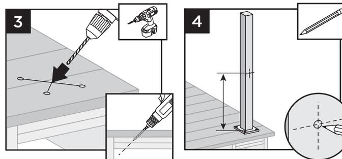
3. Using a 9/16" (14 mm) x 6" (152 mm [or longer]) drill bit, drill a diagonal hole through the decking and blocking. Ensure that the angle will allow wire to not be pinched by support plate under blocking (if using Trex ALPOSTHWDECK mounting kit).
