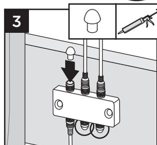
2. Attach male lead from lights to female connections on splitter. Also attach male-to-male connection wires in between each splitter. Continue until all wiring from lights are attached to splitters and connector wires are attached in between splitters.
