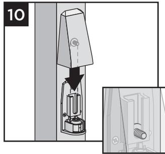
10. Slide light cover down over backing plate, adjusting mounting screws as necessary to achieve a tight fit.
