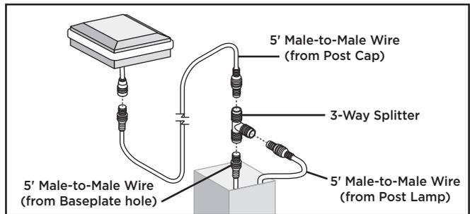
**NOTE:** If connecting a Trex® Signature™ post cap light as well, a 3-way adapter and extra 5' male-to-male wire (not provided) can be used inside the post so that only one wire must be run through the hole in the base of the post (and post blocking). This is optional.
