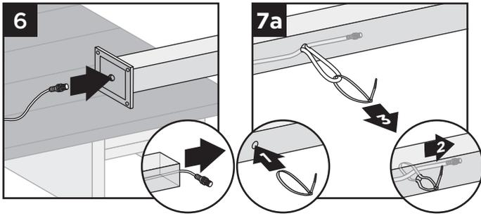
6. Turn post upside down and fish 5' male-to-male wire (provided) through hole in baseplate.
