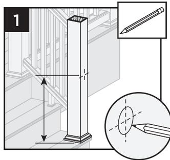
**NOTE:** If deck boards are not installed yet, place a deck board on framing to ensure post sleeve is at correct height.
