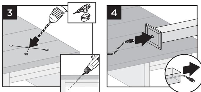
3. Using a 9/16" (14 mm) x 6" (152 mm [or longer]) drill bit, drill a diagonal hole through the decking and blocking. Ensure that the angle will allow wire to not be pinched by support plate under blocking (if using Trex ALPOSTHWDECK mounting kit). (See *Making Connections* section for details.)
