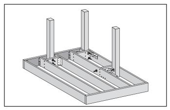
**NOTE:** To allow fascia to sit flat against framing, route/trim out back side of fascia to allow for fit over bolt locations.
