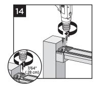
using two self-tapping screws each side (provided).
