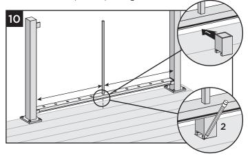
Temporarily set bottom rail into bottom brackets, and place foot block under center of bottom rail. Mark to provide placement location of base. Remove bottom rail.
