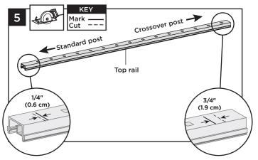
5. Top rail must be cut differently on each side of the rail. Railing side that attaches to standard post should be cut 1/4" (0.6 cm) shorter than the mark to allow for fit into top rail bracket. Railing side that attaches to the crossover post should be cut 3/4" (1.9 cm) LONGER than the mark to allow for fit into the crossover post bracket.
