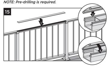
15. Attach "crowned" upper rail cover to upper rail by aligning cover on one side of rail. Then starting from one end of rail, snap cover onto opposing slot working down length of rail. **GENTLE** tapping with a **rubber** mallet may facilitate fastening.
