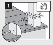
ATTACHING BRACKET. Mark with light line.
