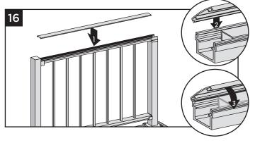
16. Attach "crowned" upper rail cover to upper rail by aligning cover on one side of rail. Then starting from one end of rail, snap cover onto opposing slot working down length of rail. In some cases, **GENTLE** tapping with a **rubber mallet** may facilitate fastening.
