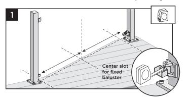
With brackets in correct swivel location, measure distance from inside of bracket to inside of bracket. ENSURE THAT BEFORE CUTTING, BALUSTERS HOLES ON BOTH BOTTOM AND TOP RAIL LINE UP. ALSO MAKE SURE CENTER BALUSTER SLOT IS AS CLOSE TO THE MIDDLE OF THE SPAN AS POSSIBLE. In some cases, due to odd railing spans, the center baluster may need to be offset in one or the other direction to ensure there is enough room at both post locations for balusters to be placed.
