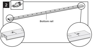
Cut bottom rail to the measurement between the bottom swivel brackets.
