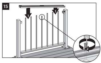
15. Working from one end of upper rail, snap balusters into upper rail working down length of rail. Fasten center baluster into center slot using two #8 x 1-1/4" (3.2 cm) screws (provided).
