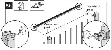
5b. When going from standard-post to crossover post, measurement must be taken from inside of top horizontal swivel bracket to inside lip of crossover
