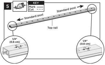
5. Cut each end of top rail 1/4" (0.6 cm) shorter than mark to allow for fit into top rail brackets.
