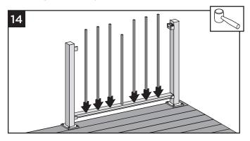
14. Place remaining balusters into holes in lower rail by snapping fully into place. In some cases, **GENTLE** tapping with a **rubber mallet** may facilitate fastening.
