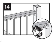
sleeves, It is not a requirement to toenail the 2x4 into the post, however if this is done predrill a hole and use a 304SS screw (not provided), that will penetrate through the aluminum sleeve.
