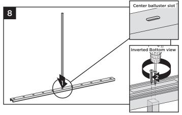
8. Attach shorter, center baluster in center slot in bottom rail using two #8  $\times$  1-1/4" (3.2 cm) screws (provided).
