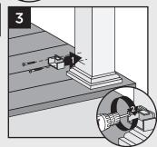
Measure up from decking surface 33-15/16" (862 cm) for 36" (92 cm) rail height or 39-15/16" (101.4 cm) for 42" (107 cm) rail height. Mark with light line.
