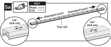
5a. Cut top rail to the measurement between the top swivel brackets. For standard post-to-standard post configurations this would be same dimensions as that of the bottom rail.
