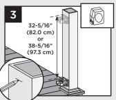
Center upper bracket on post below marked line and attach using four 2" (5.1 cm) wood screws (provided).
