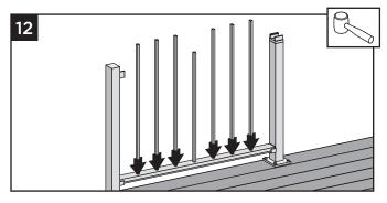
12. Place remaining balusters into holes in lower rail by snapping fully into place. In some cases, GENTLE tapping with a rubber mallet may facilitate fastening.
