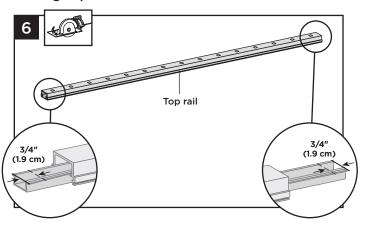
6. Slide rail insert out and cut 3/4" (1.9 cm) **FROM EACH SIDE** of insert, then slide back inside rail and center.
