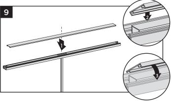
Align cover on one side of bottom rail in slot on side of rail. Then starting from one end of rail snap cover onto opposing slot working down the length of rail. In some cases, GENTLE tapping with a rubber mallet may facilitate fastening.
