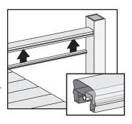
Slide baluster spacer up and snap into top rail.
