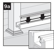
will need to be cut 2-1/2'' (64 mm) shorter than the rail to allow clearance for the RSBs on each end.
