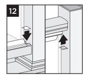
13. Attaching Post Caps and Installing Foot Blocks See instructions on page 5 and detailed foot block instructions.
