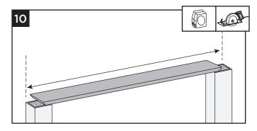
10. Cut deck boards to appropriate length of railing span, remembering to include extra space on each side of the deck board to allow for attachment to the post. Decking boards must cover 1/2 of the pressure-treated post to allow this to be fastened later. If you include extra decking material on each side, this can be cut off later if necessary.
