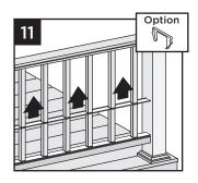
to be cut 2 1/2" (64mm) shorter than the rail to allow clearance for the RBS's on each end.
