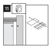
Snap spacer into bottom and top rail to hide brackets and create a seamless look.
