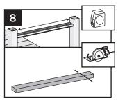
9. Place 2 x 4 on universal rail. Attach board to rail with 1-5/8" (41 mm) pan-head screws (not provided) approximately every 16" (406 mm) on center.
