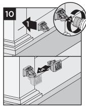
For LOWER post - install RSB FLAT SIDE UP, ABOVE MARKED LINE, using two wood screws provided. Take second RSB, turn upside down and interlock into first RSB.
