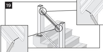
Mark both posts on inside channel of the top stair rail. Remove top stair rail. Installation Instructions
