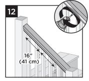
13. Slide baluster spacer up and snap into top rail.
