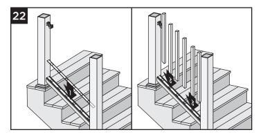
22. Place inverted top baluster spacer on bottom rail rail/ baluster spacer, ensuring that baluster holes line up. Install balusters into bottom stair rail.
