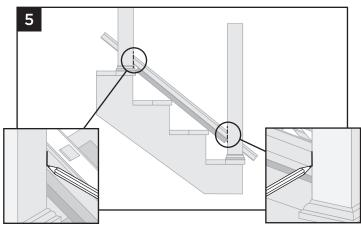
5. Use the lower and upper stair post to set the length of the bottom stair rail. Ensure that baluster spacer holes are spaced evenly between posts. Also allow for a minimum of 1-1/2" (292 mm) at each end of the stair rail for bracket placement and baluster clearance. Mark rail at post intersections.
