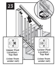
21. For LOWER post - install RSB FLAT SIDE UP BELOW MARKED LINE, using two wood screws provided. Take second RSB, turn upside down and interlock into first RSB.
