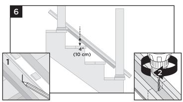
6. Mark approximate location for foot block, allowing a measurement of 4" maximum. Invert the bottom rail, and at marked location drill a hole using a 3/16" drill bit in the center of the channel. Foot block is to be installed at last step. For spans over 6' in commercial applications, mark and drill two locations spaced evenly apart for two foot blocks.
