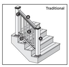
Cutting post sleeves is **NOT** required. Ensure both top and bottom post/post sleeves are tall enough to accommodate top rail and  $2 \times 4$ .
