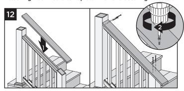
12. Place deck board on top rail and attach board to posts using two Trex recommended composite decking screws (use two screws per each post).
