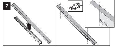
Using the cut top rail as template, cut 2x4 at same angle and length of the top rail.
