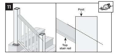
11. Cut post and post sleeves to proper angle so cut is flush with the top rail. Be careful to not cut top rail.
