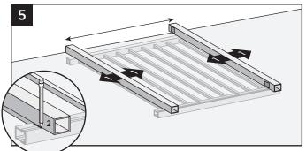
5. Adjust posts so that cut marks do not fall on a baluster. Make sure distance from first baluster to post is the same on both sides. Mark cut locations on panel.
