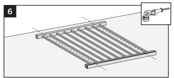
6. Cut panel using a reciprocating saw (equipped with a metal blade).
