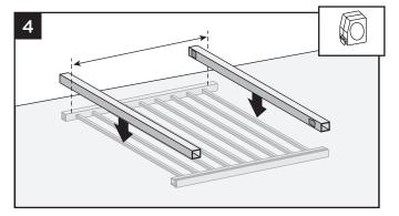
4. Lay panel on a flat non-marring surface. Place posts on top of panel. Place posts so that width measurement from Step 2 is to the outside of each post.
