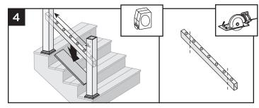
4. Set railing on top of deckboard, making sure baluster holes are vertically aligned and mark line at each intersection. When measuring, cut equal lengths from each side of railing allowing a minimum of 2" on each end from the last baluster hole to the end of the rail. This will ensure proper baluster and bracket placement and equal spacing of balusters per each railing section.
