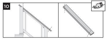
10. Measure accordingly and cut deck boards to appropriate length of railing span also allowing for additional decking material that will be installed over the lower stair rail post.
