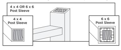
post sleeves work well for angles up to 45 degrees. Bottom rail brackets may need to be slightly offset to one side in order to fit properly to hold rail in place. Measure and mark first before attachment of bracket to rail to ensure bottom rail remains parallel to upper rail.
