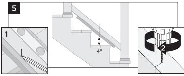
5. Mark approximate location for foot block, allowing a measurement of 4" maximum. Invert the bottom rail, and at marked location drill a hole using a 3/16" drill bit in the center of the channel. Foot block is to be installed at last step.
