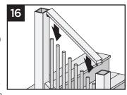
**TIP:** Pre-drill prior to screw installation using a 7/64" drill bit.
