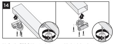
14. On the TOP RAIL, attach the assembled stair brackets to the side WITH the baluster holes. Attach both brackets using three #8-18 x 1" self-drilling screws (provided).
