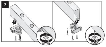
7. On the BOTTOM RAIL, attach the assembled bottom stair brackets to the OPPOSITE SIDE of the baluster holes. Attach both brackets using three #8-18 x 1" self-drilling screws (provided).
