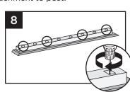
**NOTE:** A long drill bit will be required to fit inside the baluster holes.
