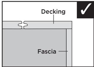
Install fascia **UNDER** decking edges/ends. This will provide protection to the fascia/framing seam as well as optimize the aesthetics of the installation.
