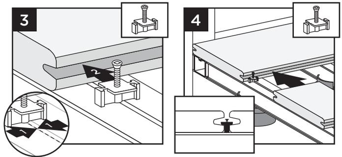
3. Insert fastener into grooved edge of deck board. Align screw hole in fastener with center of joist.
