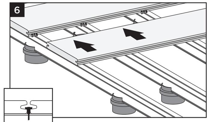
6. Slide second board into place, making sure fasteners fit into groove. Install the next universal fastener on the other side of the second board in the same manner as Steps 1 through 5.
