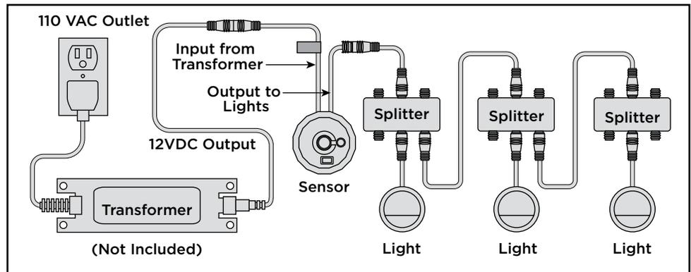
**Note:** Make sure the sensor is installed after the transformer, but before the first light. Any lights that are installed before the sensor will not be controlled.
