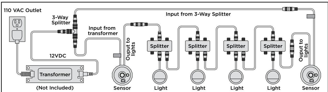
To install two sensors, place a motion sensor at each end of the circuit, making sure you connect the wire with the red tab to the transformer side of each circuit.
