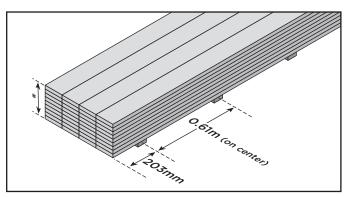
\*Enhance decking, and 1 x 12 and 1 x 8 products: maximum stack height is 12 bundles. Transcend decking: maximum stack height is 14 bundles.
