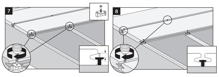
Installing Last Deck Board (Square-Edge Board Recommended)
