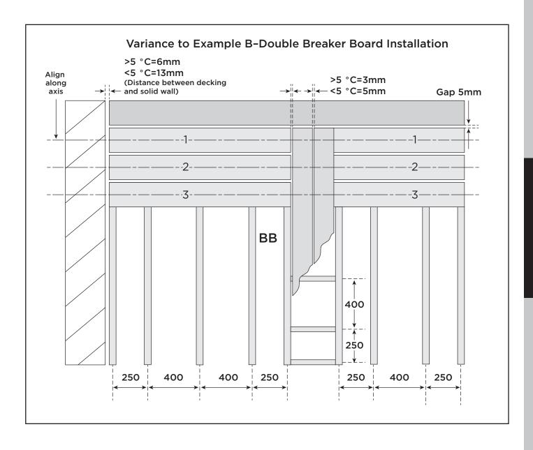
IMPORTANT: Each board end must rest on a separate sub-framing member and be attached with two universal fasteners or screws each! All sub-framing must be attached to the ground or secured by appropriate aluminum frame brackets as per previous examples.
