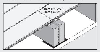
**NOTE:** Optional - Gap joist framing 3mm - 6mm to allow for water drainage.
