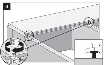
**NOTE:** Use scrap piece of decking to help hold fastener in place while attaching.
