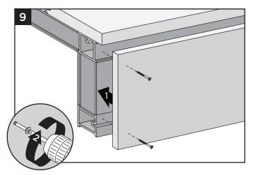
**NOTE:** Fascia wider than 60mm will require more detailed fastener requirements. Fascia boards are not allowed to carry loads from decking. Contact a Trex representative for more detail.
