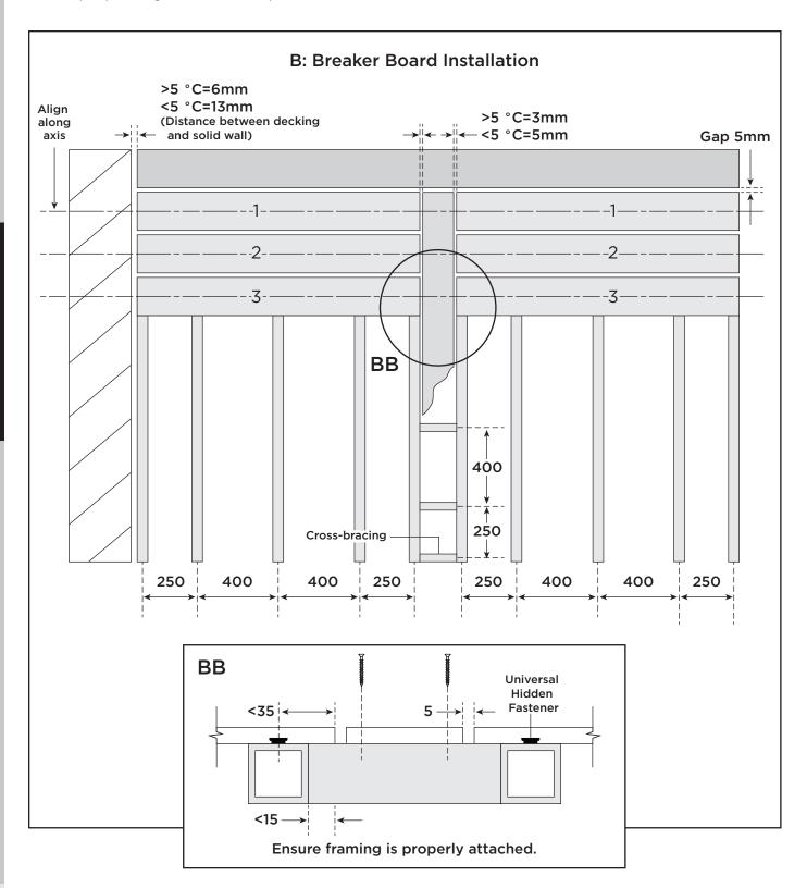
To obtain a continuous joint pattern, boards must be averaged to their longitudinal axes!
