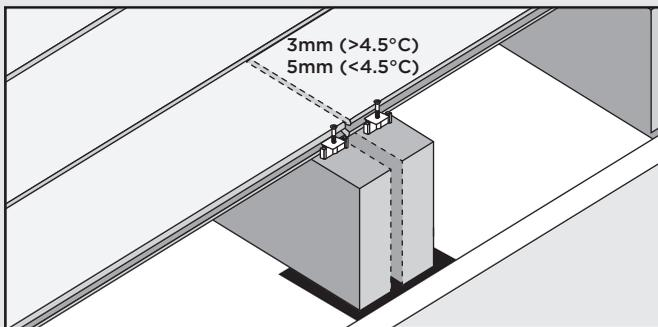
**NOTE:** Optional - Gap joist framing 3mm - 6mm to allow for water drainage.
