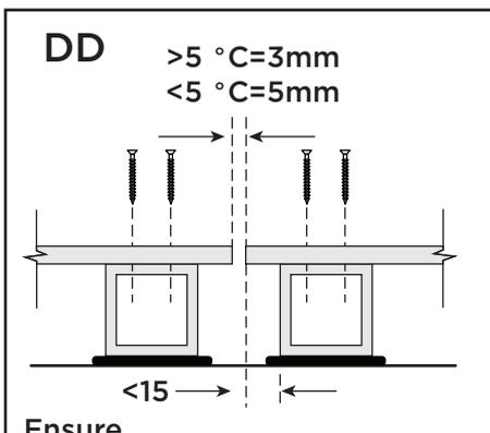
Ensure framing is properly attached
