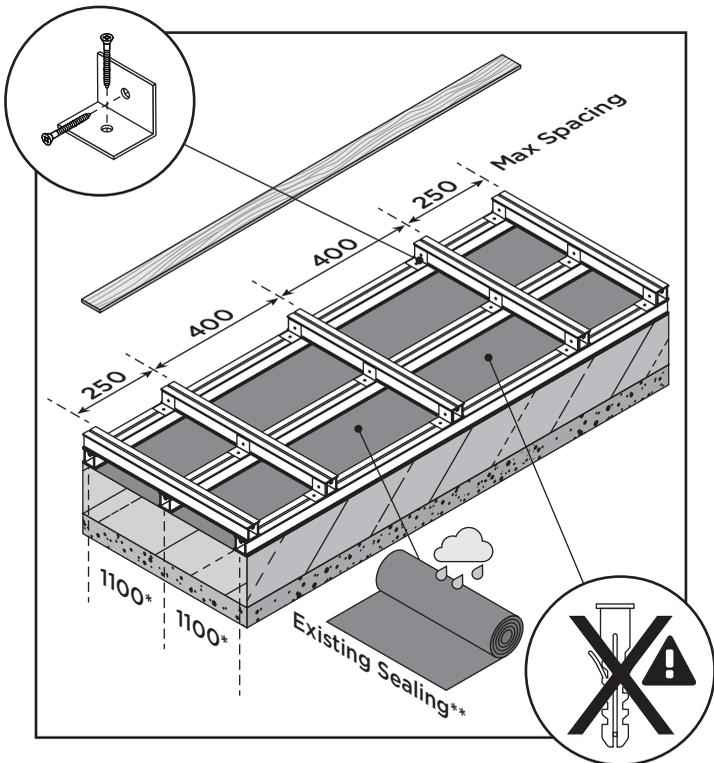
\* Reinforcement or counter spacing depends on the supplier and the aluminum dimensions.
