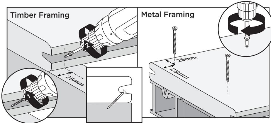
For timber framing, and if using Trex Universal Hidden Fasteners, pre-drill and toenail an approved screw at an angle in groove at both ends 25mm from board end and center of each board.
