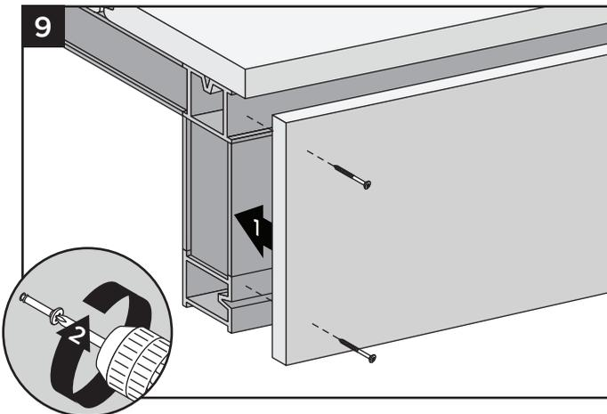
**NOTE:** Fascia wider than 60mm will require more detailed fastener requirements. Fascia boards are not allowed to carry loads from decking. Contact a Trex representative for more detail.
