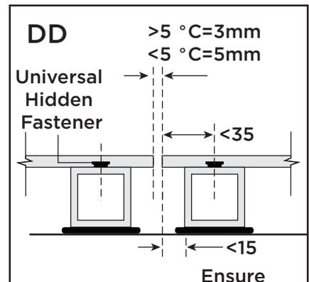
Ensure framing is properly attached
