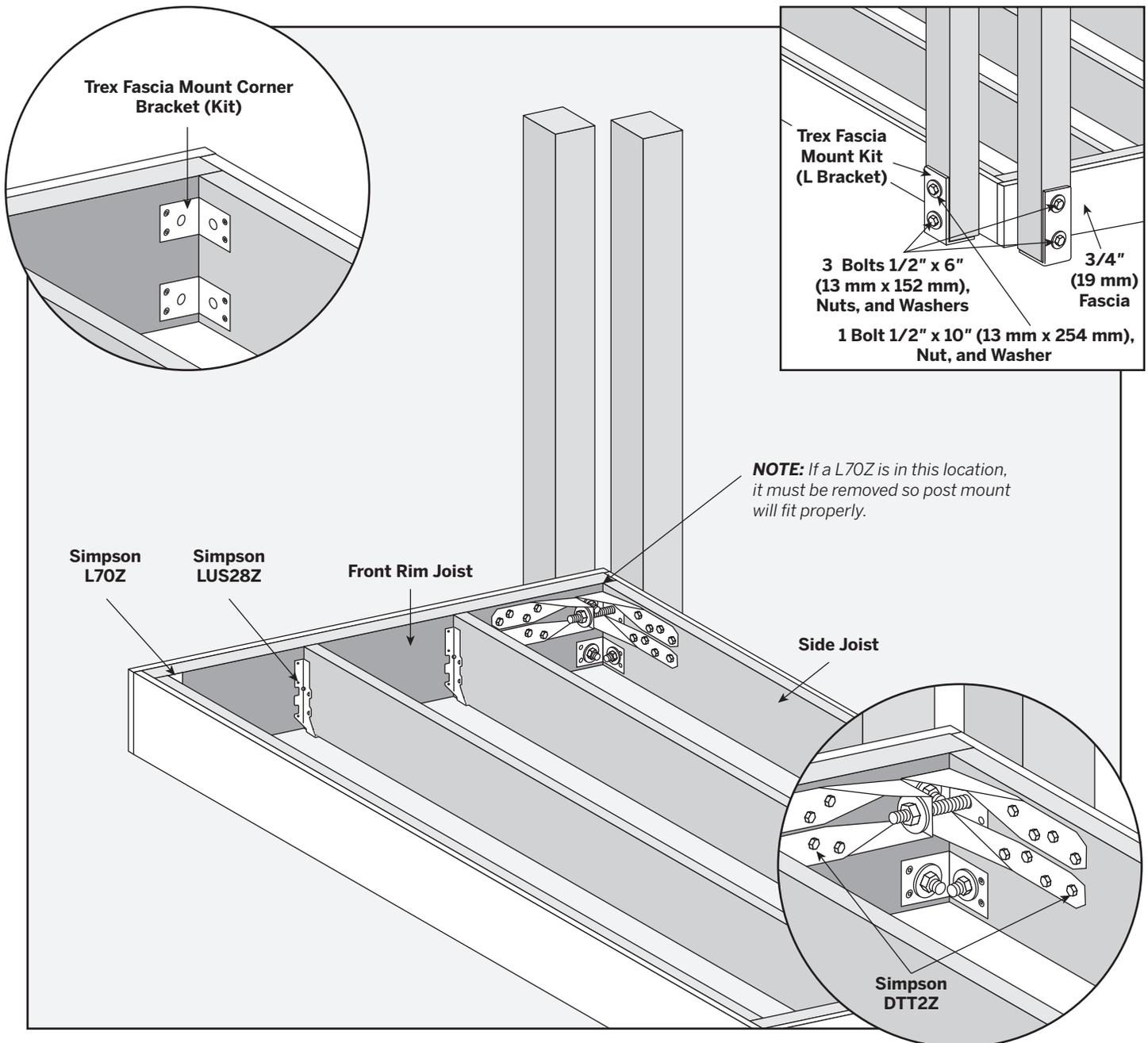
1. Install post on rim joist and fully tighten using Simpson DTT2Z on top bolt.
