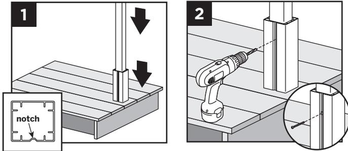
6. Place or rest bottom aluminum guide block on bottom of post. Place guide on post so that notch is on a side that does not require railing to be attached.
