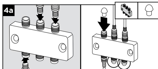
4a. Use male-to-male extension cables to make connections to splitters (*all sold separately*). Cap off all unused female connections on splitters using caps provided or weather resistant silicone.
