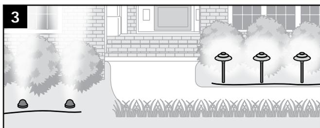
3. Run all wires from the power source locations to the lights on top of the soil, being mindful to leave slack. Pay special attention if using separate circuits with independent dimmers (grouping lights by type is recommended).
