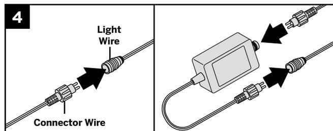
4. Connect all lights. Wire the optional dimmer (recommended) between the main 20' (6.1 m) transformer to male lead and the transformer for each circuit. Ensure connections (including splitters), fixtures, and power sources all work properly.
