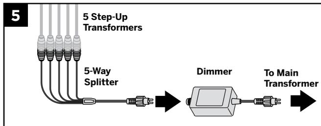
5. If using an optional dimmer (recommended), simply place the dimmer between the 5-way splitter and main transformer.
