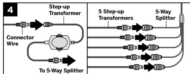
4. Connect opposite end of male connector wire cable to female end on Step-up Transformer. If using more than one spotlight, use 5-way splitter on Step-up Transformer, making sure that each spotlight is utilizing its own 36V Step-up Transformer. Wire the Step-up Transformer or 5-way splitter to the 5A main transformer.
