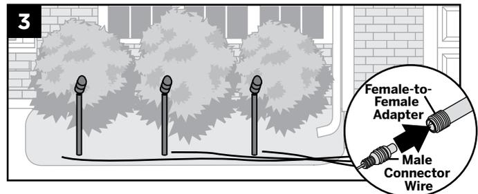
3. Connect opposite end of female adaptor to male connector wire. Choose appropriate length wire based on your needs. Run all wire on the surface back to the location of the power supply.
