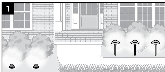
1. Locate placement of lights and lead wiring. Plan accordingly if you choose to bury wire under concrete or other permanent structures.
