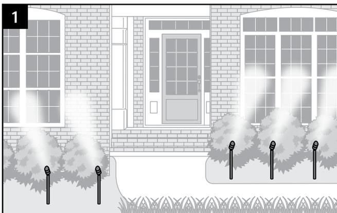
1. Locate placement of spotlights and lead wiring. Plan accordingly if you choose to bury wire under concrete or other permanent structures.
