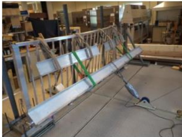
Photo No. 2 Uniform Test Load at 45°
